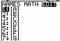
The [A], [B], [C], ... are all "variables" into which you can store different matrices. If you want to put the matrix into [A], highlight "[A]" and hit [ENTER]; if you want to put the matrix into [B], use the down arrow to highlight "[B]" and hit [ENTER]; etc. For this example, we will put the matrix into [A], so hit [ENTER]. You will see
